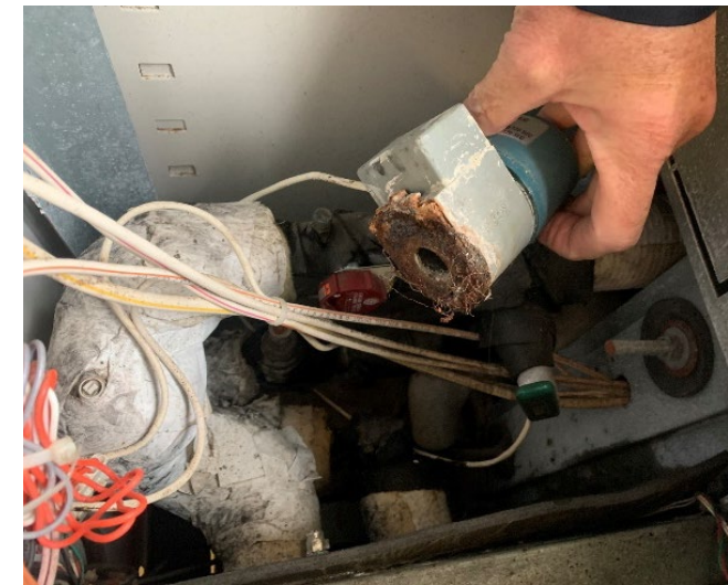
FAILED UNIT VENTILATOR ACTUATOR
